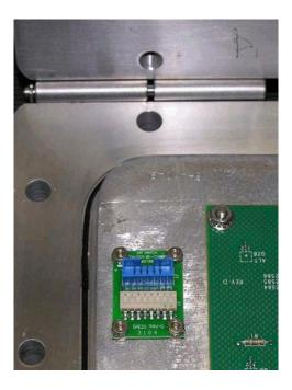
Figure G-2. Explosion-Proof Controller DIP Switch
