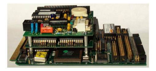
Figure 2-6. CPU Board with Modem and COM4A Piggy-Back Board
