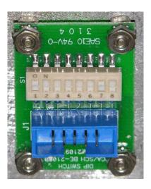
Figure 3-8. COM ID DIP Switch
